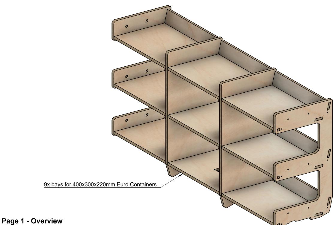
All units in mm Plywood thickness = 12mm
