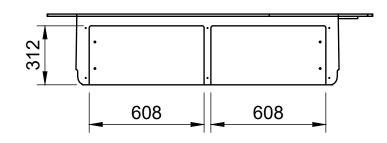
All units in mm Plywood thickness = 12mm YOKE VANS info@yoke-van-kits.co.uk 0208 132 9221
